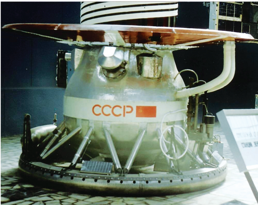
Figure 1: General view of the Venera-13, -14 and Vega-2 Landers. The Soil Sampling System is seen on the right side over the dampening torus. The vacuum tank of the Soil Sampling System is seen over the dampening torus on the left side
