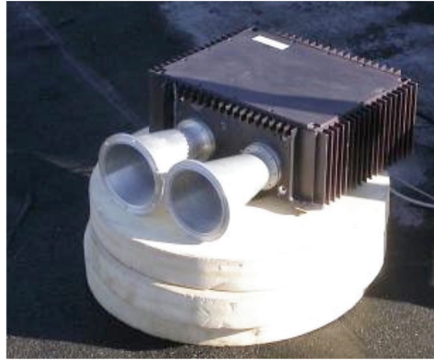
Figure 4: Two-channel prototype of the radiometer during field tests
