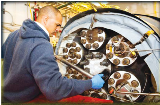
Figure 2: Testing in GEER at Venus surface conditions
